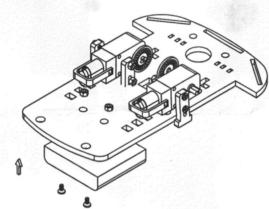
Step4:插入螺丝,固定电池盒 Step4:Insert the screws and fix the battery container
