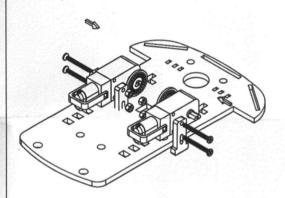
Step3:插入螺丝,把电机固定到小车底板,并拧上螺帽 Step3:Fix the motor to the chassis,then insert and tighten the screws.
