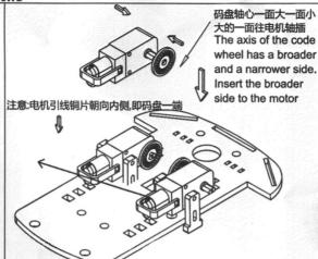
Setp2:Install the code wheel and fix the motor to the chassis.(Attention,the copper sheet of the leading wire of the motor should face inside,the same side of the encoder)
